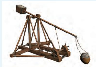
Trebuchet - Uses Counterweight
